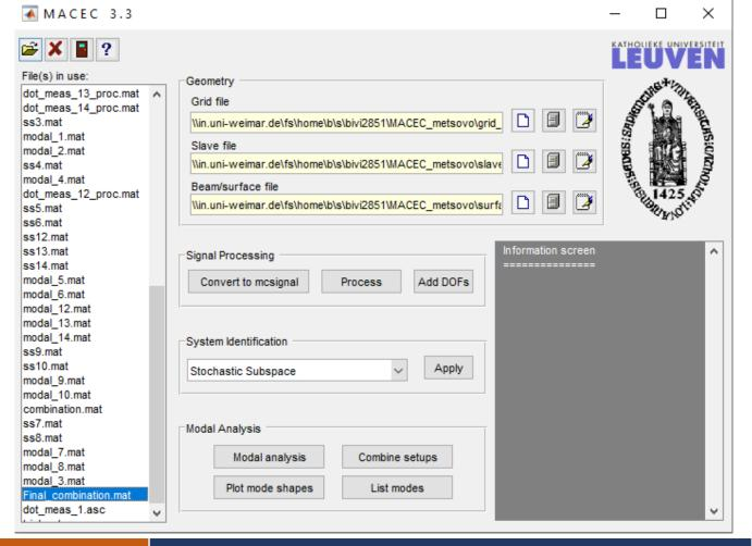
Geometry Definition Signal Processing System Identification Modal Analysis Results
