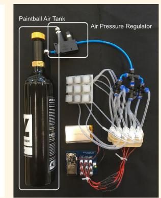
The system of high-pressure air tank not only provides air, but also reusability, mobility, and immersive experience for the user due to air regulators, refilling, lighter weight, and lower noise.
