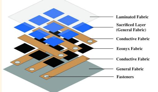
The Hug Sensor detects haptic pressure using a Pressure Sensor Matrix (resistive sensors) built from several layers of E-textile.
