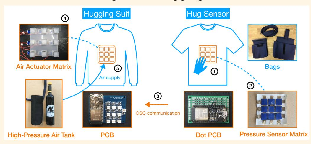
1. The hugger hugs and touches the Hug Sensor. 2. Pressure Sensor senses the hugs. 3. PCB collects and transmits the signal wirelessly. 4. The PCB controls the air valves of air actuators. 5. Inflated and deflated actuators simulate hugs and touches on the hug receiver.
