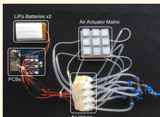
The haptic interface on the Hugging Suit provides pixelated haptic simulations with an Air Actuator Matrix (pneumatic actuators), which was created from customized silicone. The structure of McKibben artificial muscle and two-point discrimination values are utilized in the design.
