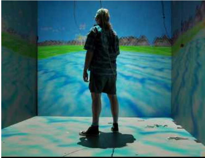
Figure 47. Cruz-Neira's CAVE. Within the system, the user's head position is tracked so that what is displayed preserves proper perspective in adapting to movements and change of location of gaze.
