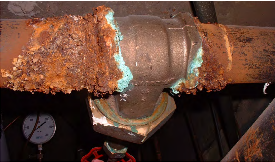
Figure 4: Iron reaction to brass. Photo credit: Corrvew.
