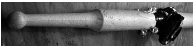
Illustration 2: drum stick with four infrared LEDs
