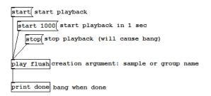
The play (or dplay) object is the basic mechanism for audio playback in EApd. It takes either a sample name or a group name as a creation argument. A bang is output when sample playback is complete.
