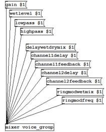
The mixer object is an object that can send messages to audio channel/bus effects as well as groups of sounds defined in the spore audio system (as opposed to groups defined in EApd itself). This is used to do mix automation of volume levels and effects based on game input.
