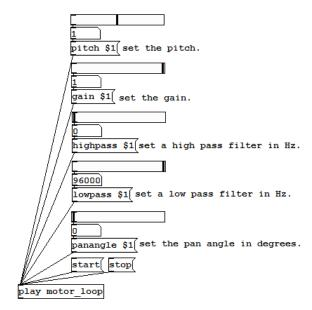
The parameters of the play/dplay objects; this is the basic set available. Not shown here are the x/y/z positional parameters used for 3d sounds.
