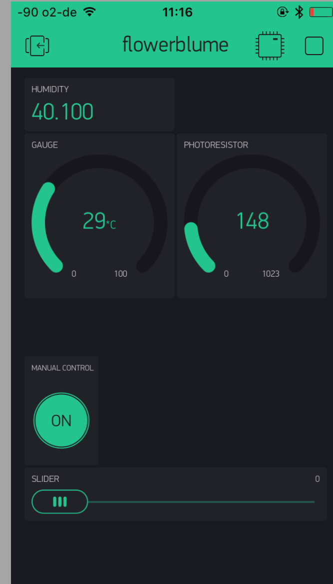
For now flowerblume can be controlled manually by Blynk. It also shows real time data from the sensors.
