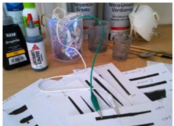
Self-made conductive ink by Pavel Karpashevich
