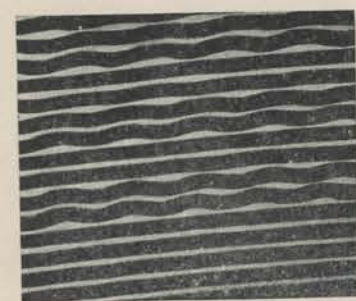
5. Surface aspect. Caruso's "high" c on a phonograph record. Microphotograph.
