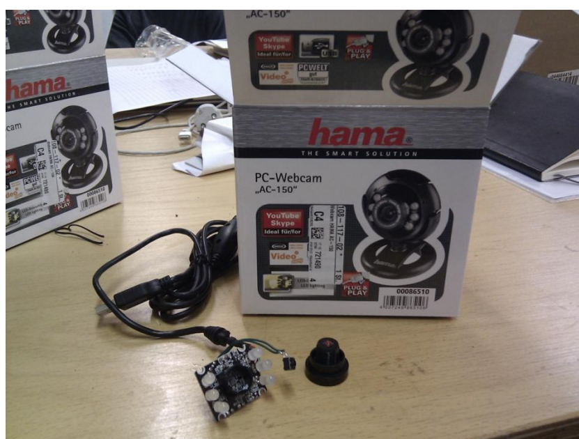
Image 1. The disassembled camera in front of the original package.
