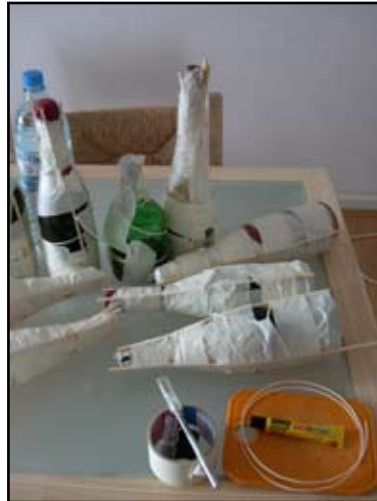
Forming the balsa wood on wine bottles and finished wood ready to be put together.
