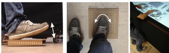
Figure 6: Augmented DJ application with feet gestures recognized by audio DTW analysis [4].
