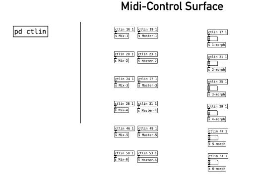
The midi-control surface, which is hidden in a subpatch, is the location where most of the midi input channels (ctlin ...) are routed to send objects. The receive objects fitting the send objects can be found patched to the switches and faders that are meant to be midi controlled.
