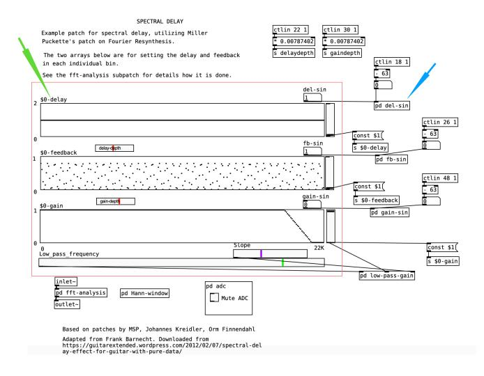
In this subpatch another subpatch called "pd adc" can be found, which contains the audio input (adc~) of the piezo mic.
