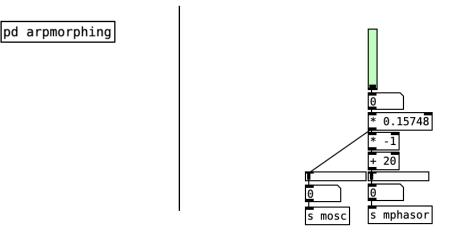
The crossfader (coloured green) is receives the midi control information from the Midi-Control Surface and outputs values from 0 to 127. Both volume faders (coloured white), that are connected to the oscillators via the send modules work with values from 0 to 20, so the first step is to send the values through the "\* 0.15748" object, that translates them to values from 0 to 20.
