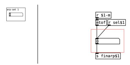
Here we can find the receivers of the select object of the arpeggiator, called "r sel\$1". The "\$1" is defined by the numbers 1 to 6, given to the six subpatches. We can also find a receive object called "r \$1-m". This object recieves midi notes from the 6 Oscillator Modules shown above. (read about it on page 15) These midi notes are changed to a number resembling a Hertz frequency in the mtof object. (mtof = "midi to frequency")
