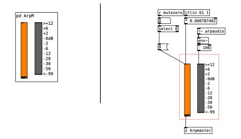
The master volume fader has multiple value inputs. One of the inputs is the receiver of the on/off toggle of the Arpeggiator Module. It sends the value 0 to the master volume fader, as already mentioned above. The other value input is the midi control input. This volume fader works with the values 0 to 0.1, so the this time the multiplication object "\* 0.000787402" is needed to translate the values given by the midi input.
