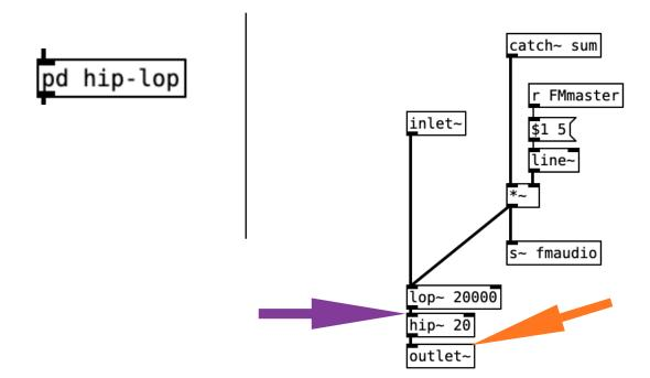
This subpatch is the exact place, where the audio signal of the arpeggiator and the 6 Oscillator Modules join together. The audio of the oscillator modules is volume controlled by "r FMmaster", which receives values from the Master Volume Control.
