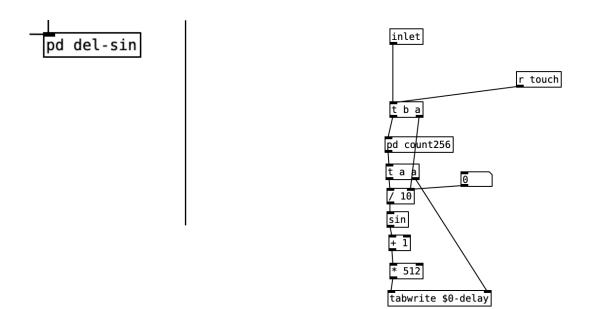
Here the number signal of the piezo input is received by "r touch" and intervenes in the "t b a" object, which is a part of the system, that writes the sine frequency in the spectral delay array. (marked with a green arrow in the delay subpatch)
