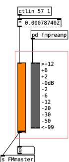
It works exactly like the master fader of the arpeggiator, but receives its own midi control values, so the volume of the arpeggiator and the oscillator modules do not depend from one another.
