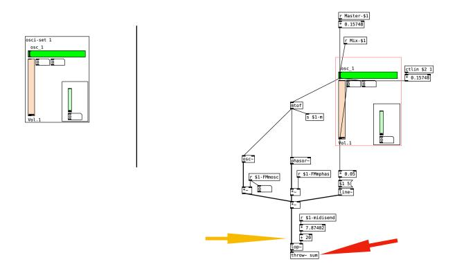
The 6 oscillator modules, that can be used as for frequency modulation synthesis, are basically 6 oscillators with 3 different parameters that can be controlled: Hertz frequency of the oscillating wave, volume/amplitude of the wave, and a crossfade between sine wave and sawtooth wave.
