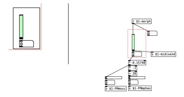
The midi control comes from the Midi-Control Surface and is received through "r \$1-morph". These midi notes are translated to the correct crossfader values, and they are also transmitted to a lowpass filter via "s \$1-midisend".
