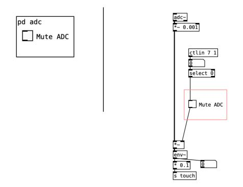
The audio input ("adc~") receives the audio signal from the piezo microphone. It is amplified with the value 0.001 and can be muted with a midi controlled toggle, working the same way as the on/off toggle of the arpeggiator. The audio signal is translated into a number signal via an "env~" object and sent ("s touch") to the subpatch "pd del-sin" that can be found in the delay subpatch. (marked with a blue arrow)
