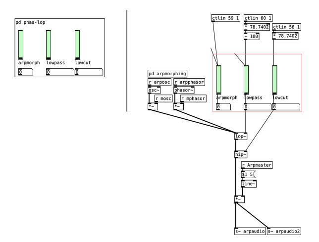
The Arpeggiator-Filter Module is the first part of the arpeggiator system, where audio comes into play. But the module does not only contain the oscillators of the arpeggiator, it also contains the most parameters and filters that are shaping the sound of the arpeggiator.
