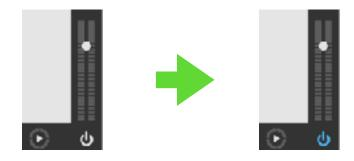
Now you should hear an audio signal and the two bars close to audio on/off button you just pressed should project some volume (light up too).
