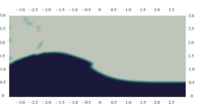
Figure 7c: Simulation snapshot of the liquid damper at the time instant of 120 s (see Fig. 7b).
