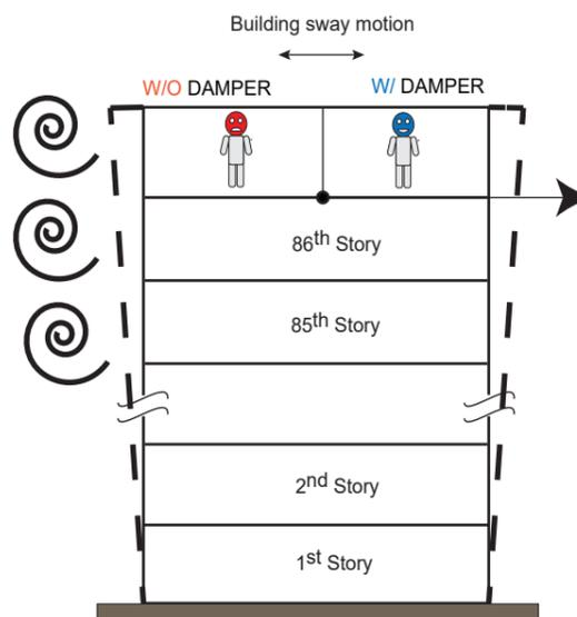
Figure 7a: Schematic representation of a building subjected to sway motions caused by high wind speeds. Left side: Case without damper Right side: Case with damper.
