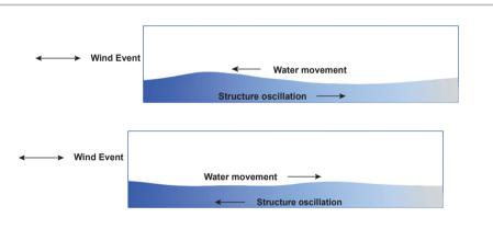
Figure 5: Simulation of water behavior inside a tank, subjected to an horizontal motion
