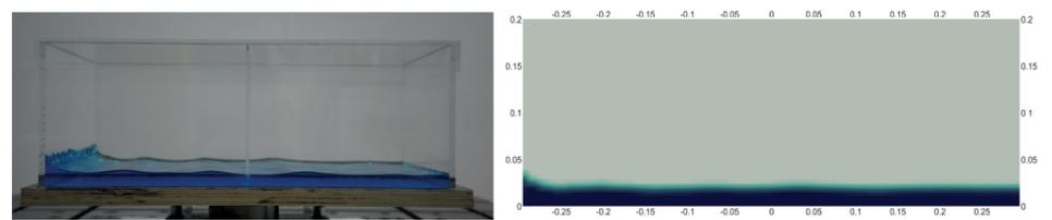
Figure 6: (left) Sloshing experiment at shaking table at Geotechnical Department of BUW / (right) Numerical sloshing under similar excitation conditions and geometry [3].
