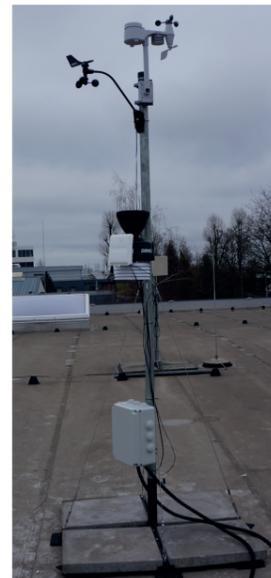
Figure 3: Weather station deployed on the top of a roof (industrial building). Long-term measurements for climate observations (wind speed, temperature, precipitation, humidity).
