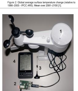
Figure 4: Measurement system for weather station 1 - Weather station (Bresser 6in1), 2 - Raspberry Pi with Raspyre framework [2], 3 - Antenna USB connection, 4 -Weather display.
