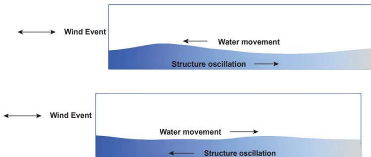
Figure 5: Simulation of water behavior inside a tank, subjected to an horizontal motion.
