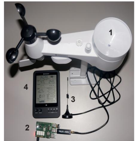
Figure 4: Measurement system for weather station 1 - Weather station (Bresser 6in1), 2 - Raspberry Pi with Rasperry framework [2], 3 - Antenna USB connection, 4 - Weather display.
