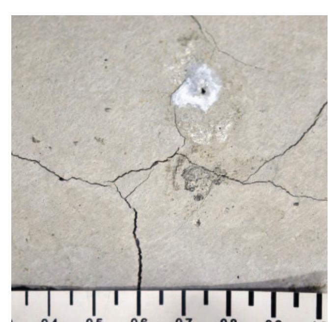
Fig. 1: Crack and gel formation after ASR [o. i.]
