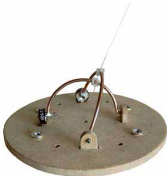
Figure 1. The Vectorix unit: 1 - string, 2 – metal brackets, 3 - rotary potentiometer
