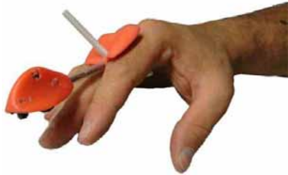
Figure 4. The Mosca device. Pointer and middle finger grab the front part of the device and the thumb manipulates a mini-joystick and a mouse wheel.
