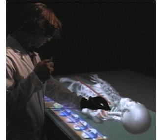
Figure 6: The zoom tool: The left hand positions the skeleton and provides the focal point, while the right hand zooms in by moving away from the focal point. Similarly, one can zoom out by moving the left hand towards the focal point.
