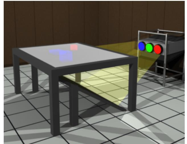
Figure 2: The Responsive Workbench. A video projector projects a high resolution stereoscopic image through a mirror onto the table top. The system is currently driven by a Silicon Graphics Onyx RealityEngine2 graphics system at a resolution of 1025x768 pixels at 96Hz, 48Hz per eye.
