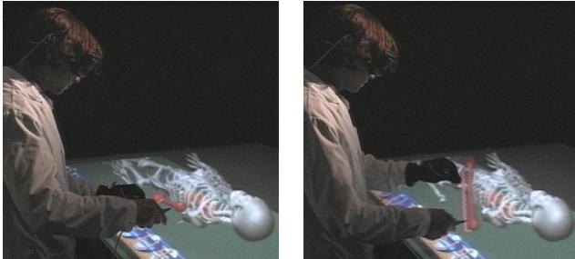
Figure 9: The grab-and-twirl tool. The user first grabs an object with either hand and manipulates the object as a one-handed 6 DOF grab. At some point, the user pins the object with the other hand and performs a symmetric object twirl. Thus the user experiences a non-explicit transition between a one-handed grab and a two-handed grab.
