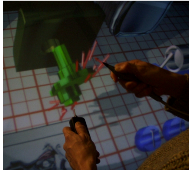
Figure 1. Two hands are used to fit the crankshaft into the bearing.
