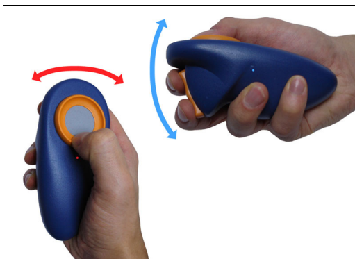
Figure 3: Using the gyroscopic rotation sensor to indicate directions
