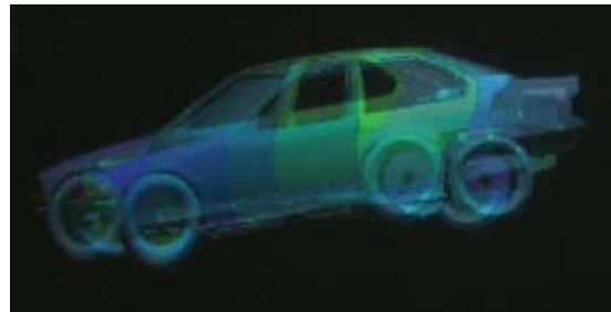
Figure 8. An image taken directly from the projection screen. It shows four images overlaid on top of each other. Two images are displayed for the left user's eyes and the other two images for the right user's eyes.
