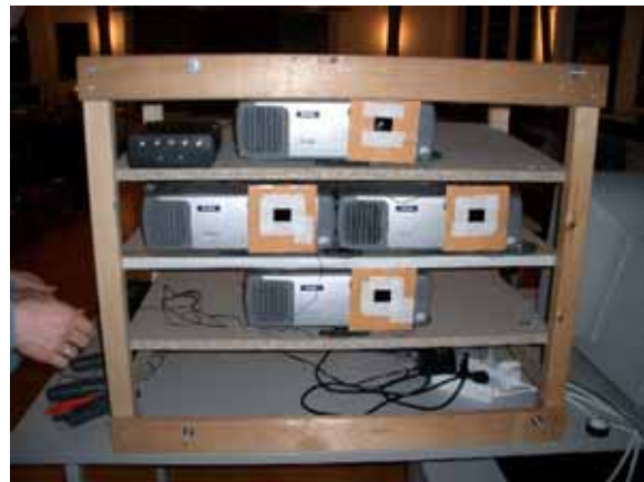
Figure 1: Four shuttered LCD projectors. Small shutters are mounted in front of each projector.
