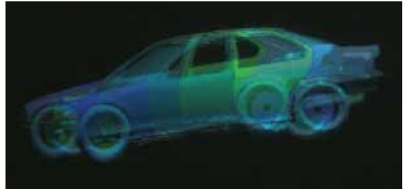
Figure 4: An image taken directly from the projection screen. It shows four images overlaid on top of each other. Two images are displayed for the left user's eyes and the other two images for the right user's eyes.
