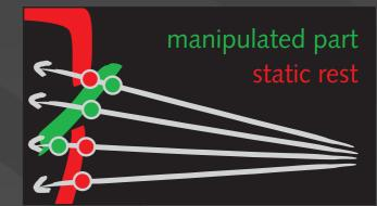
lighting computation for the intersection closer to the reflecting surface (in case there are two possible)
