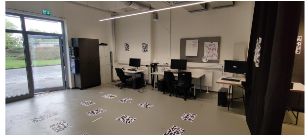
Figure 4: Image of the study room with the markers placed to act as feature points to improve ARCore’s tracking.
