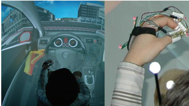
**Figure 1:** User interacting with a virtual car interior in the CAVE (left), finger tracking system with our tactile feedback device at the user's hand (right)
