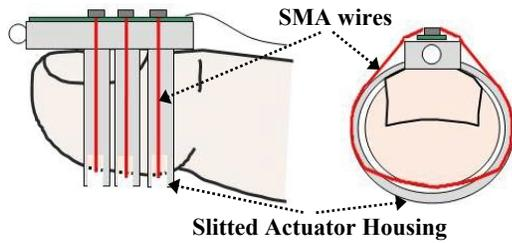
**Figure 2: Schematic view of a thimble device**
