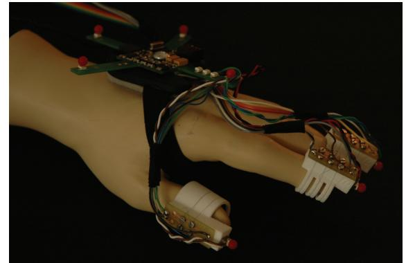
**Figure 4: Final prototype of our tactile feedback system combined with the finger tracking system by A.R.T.**
