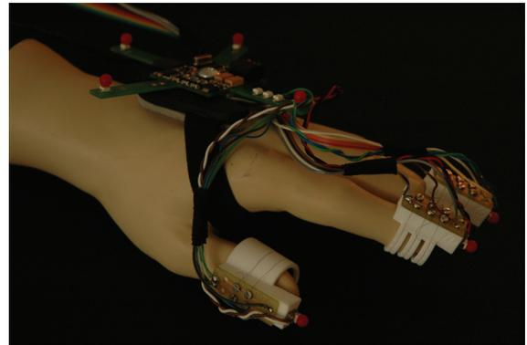
**Figure 4: Final prototype of our tactile feedback system combined with the finger tracking system by A.R.T.**
