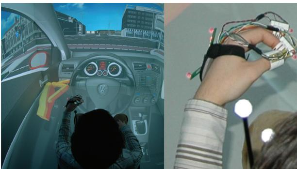
Figure 1: User interacting with a virtual car interior in the CAVE (left), finger tracking system with our tactile feedback device at the user's hand (right)
