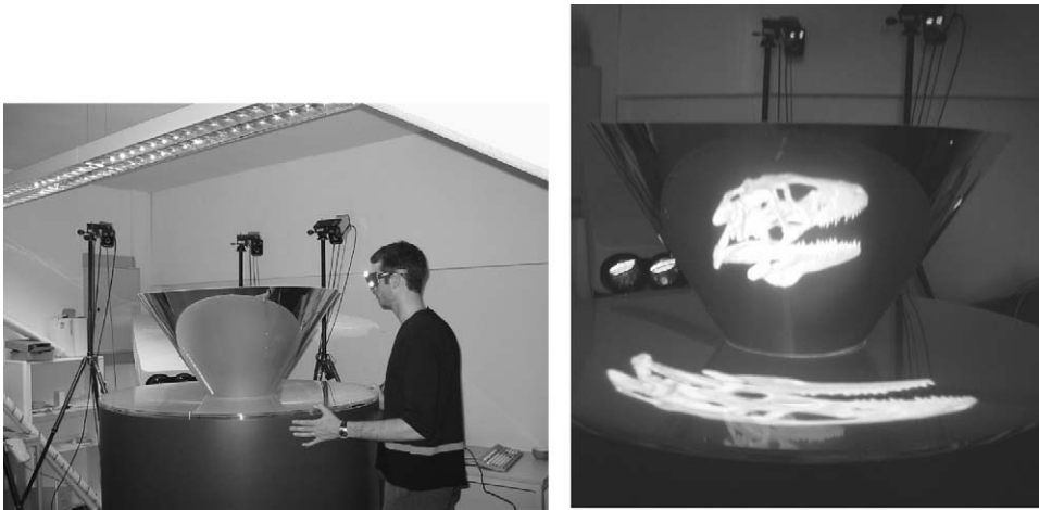
Fig. 1. A head-tracked user (left) observes a warped image (right) inside the Virtual Showcase.
