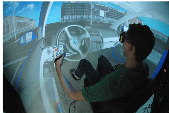
Figure 1: A user interacting with a virtual car interior in a projection-based immersive environment
