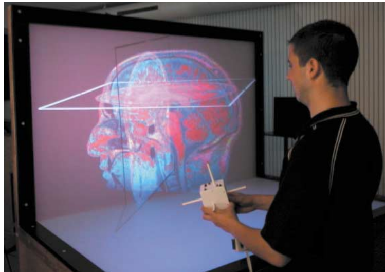
2 Using the Cubic Mouse to control three orthogonal cross sections through an MRI data set of a human head.
