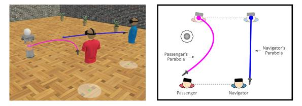
Figure 1: Target specification with *Multi-Ray Jumping* for two collocated users. While the navigator (blue shirt, right side) specifies a target using the blue parabola, the magenta curve adjusts accordingly to show the offset target location of the passenger (red shirt, left side). The initial direction of the magenta curve is defined by the passenger's controller.
