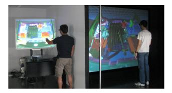
Figure 8: The test setup used in the second experiment. Both users were sharing the same virtual environment consisting of a car's engine compartment. They were operating on two different systems standing in close proximity, but not allowing direct visual contact. The *presenter* was using a smaller screen (left side) then the *observer* (right side).
