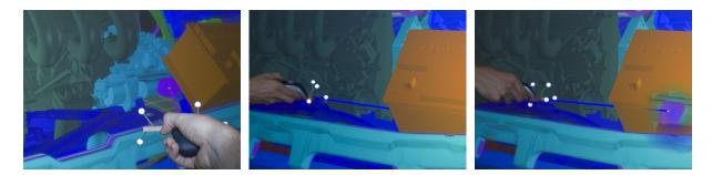
Figure 1: The first two images (a, b) illustrate the issue of interpersonal occlusion between two tracked users in a multi-user VR system: an object that is fully visible to one user (a) cannot or only partially be seen from other viewpoints (b). Show-through techniques can improve target discovery in such situations by showing the indicated object through the occluding environment (c).
