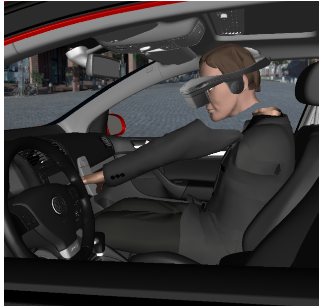
Figure 7: When the user leans forward and stretches his arm in order to reach the navigation system the simplified body model produces gaps between the moving body parts and the fix torso.
