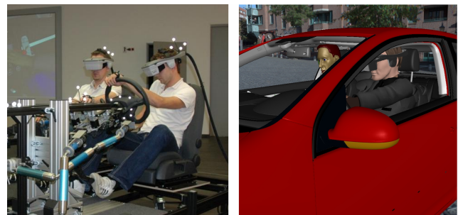
Figure 1: The two-user seating buck scenario. The image on the left side shows the hardware setup. The right side shows the same perspective for the virtual car model including the two avatars.
