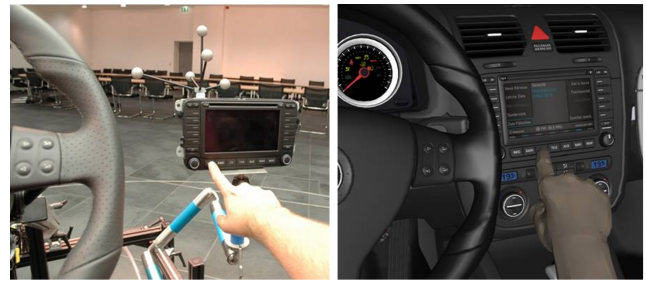
Figure 3: On the left side the navigation system panel mounted on an arm of the flexi-holder is shown and on the right side the corresponding virtual image through the driver's HMD.
