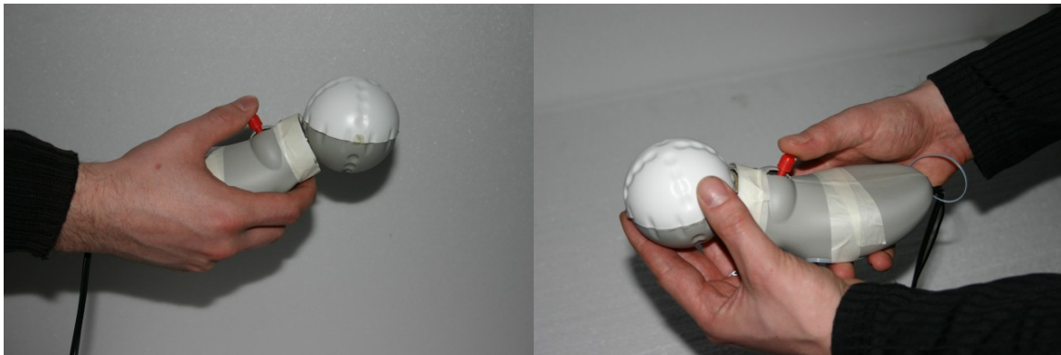
Figure 5: An actual prototype of the device in Figure 4. The device consists of a two axis gyroscope inside the handle, a 1-DOF joystick operated by the thumb, and 3-DOF joystick inside the ball.
