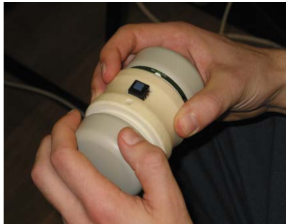
Figure 3: The YoYo consists of two SpaceMouse sensors attached to a grip in the middle
