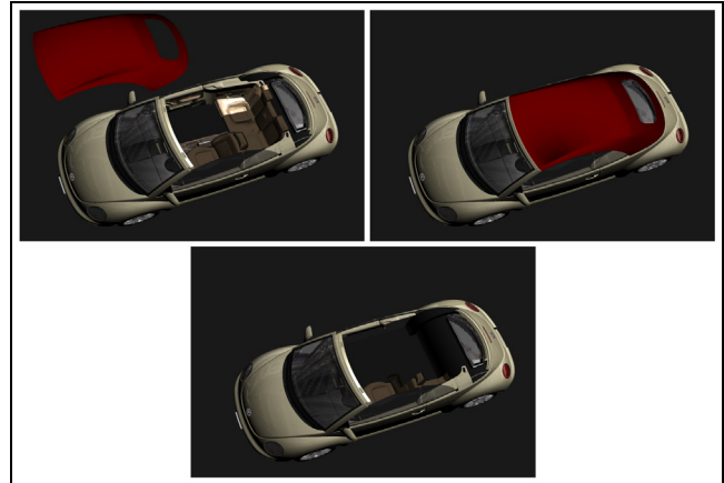
Figure 1: The algorithm allows manipulations of arbitrary objects in the scene without losing the occlusion culling ability. In the upper images you can see how the marked roof is translated by the user. The lower image shows that interior parts of the car are missing, since they would be occluded by the roof (not displayed). (Note: The original model does not have a second front seat!)
