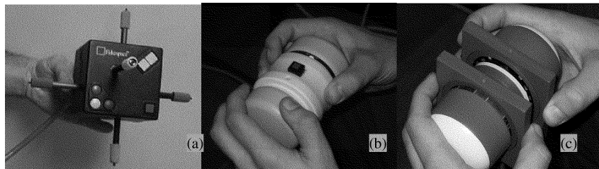
Fig. 1. (a) The CubicMouse is commercially available. The cube-shaped box is held with the non-dominant hand, while the dominant hand manipulates the rods. (b) The YoYo consists of two SpaceMouse sensors attached to a handle in the middle. (c) The SquareBone's handles attached to the contained SpaceMouse sensors can be simultaneously manipulated with the finger tips.
