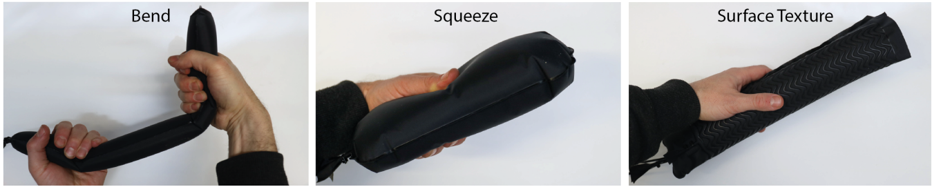
Figure 4: The three inflatable prototypes controlled with pneuCNTRL . Each represents the data through a different haptic feedback: Bend (low pressure values are easy and high values difficult to bend); Squeeze represents data through the resistance felt when squeezing the artifact; for Surface Texture, a texture can be felt at higher pressure values, but it disappears at low values.
