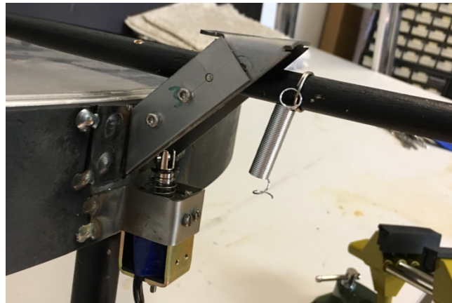
Figure 3: Detail of the mechanics with solenoid.
