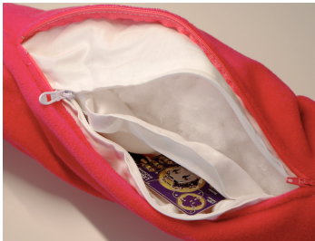
Figure 5: Electronics are hidden but still easily accessible for maintenance.
