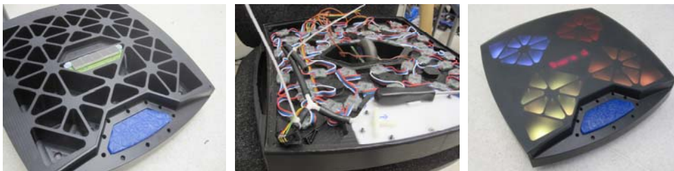
Figure 1: The CNC machined PlazaPuck with low and higher resolution display, pressure pad and wheel.
