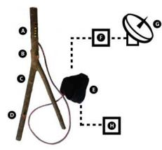
Figure 3. Solar Radiation Dowsing Rod system design. (A) LED strip (red, orange, green), (B) embedded IMU module, (C) two embedded 5v vibration motors, (D) push button, (E) armband pack including a microcontroller, 9v battery, wireless radio frequency module, (F) PC connected to telescope, (G) 2-meter radio telescope with 2.4GHz receiver, (H) COSM Server.
