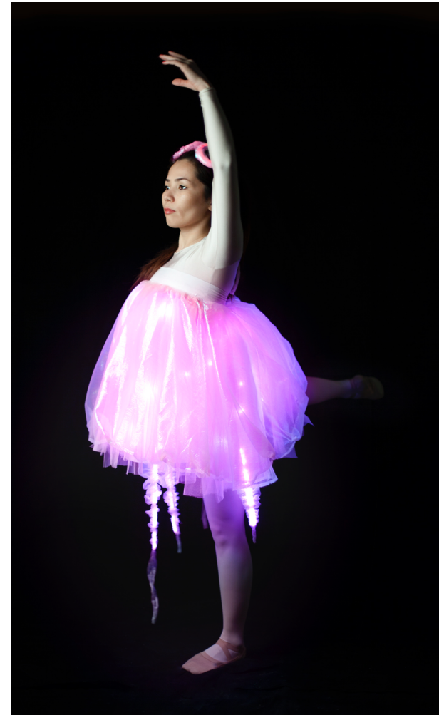
Figure 7. The Jellyfish, pulsating in white when standing still. The balloon dress turns red for a moment if the dancer is twisting, the tentacles underneath turn red in response to up-down arm movements.
