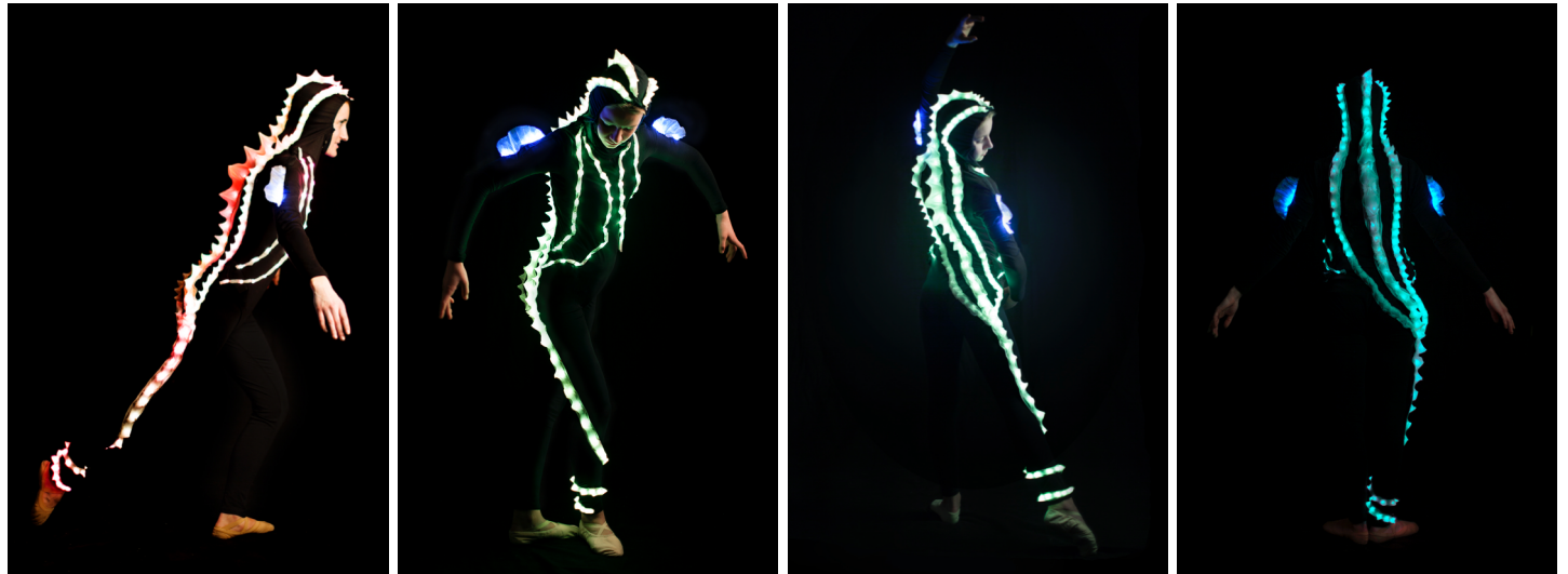
Figure 2. The Seahorse costume in action, changing colors according to sensed motion (velocity, arm movements, and twists).
