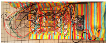
Figure 12: Integrated connections from pages to spine.
