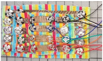
Figure 11: Close-up of the three different layers with conductive fabric and snap fasteners for each circuit.
