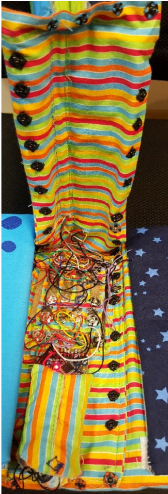
Figure 9: Book spine with micro-controller and connections from individual pages.
