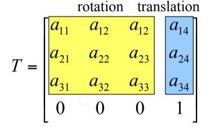
will always be the result of the successive application of a 3x3 rotation matrix and of a translation (if the body is rigid)
