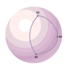
The figure shows that if we have an intermediate position q2, the interpolation from q1→q2→q3 will not necessarily follow the same path as the q1→q3 interpolation.
