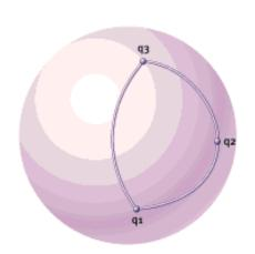
• The figure shows that if we have an intermediate position q2, the interpolation from  $q1 \rightarrow q2 \rightarrow q3$  will not necessarily follow the same path as the  $q1 \rightarrow q3$  interpolation.
