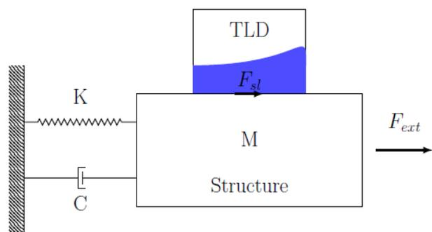
Equivalent mechanical model of spring-mass-dashpot with tuned liquid damper
