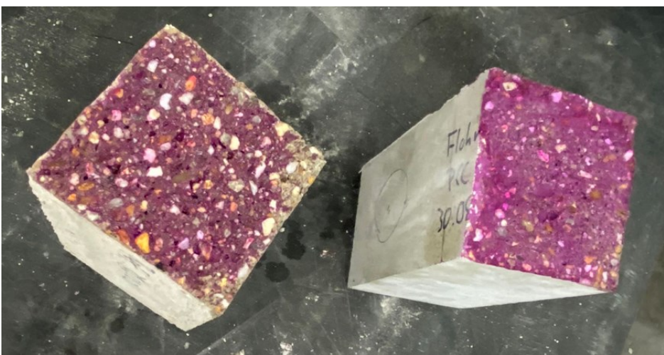
Fig. 3# carbonatization depth of PCC vs. CC
