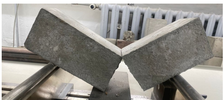
Fig. 6# flexural strength test
