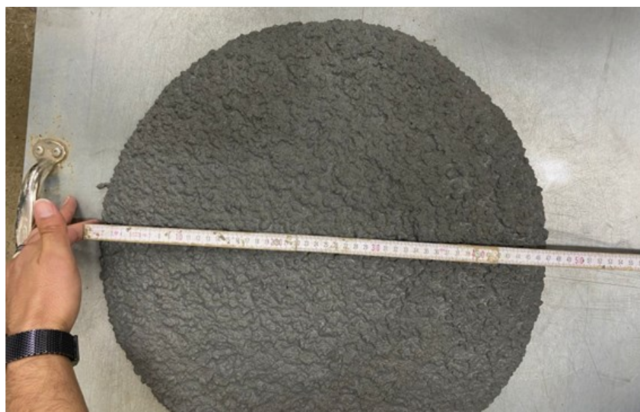
Fig. 5# spread flow (flowtabletest)
