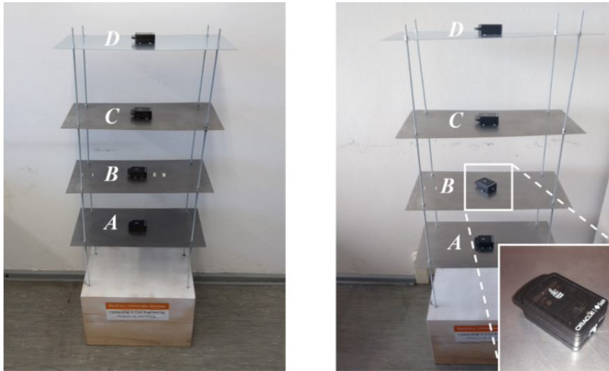
Figure 6: (a) Laboratory test setup and (b) simulated sensor fault
