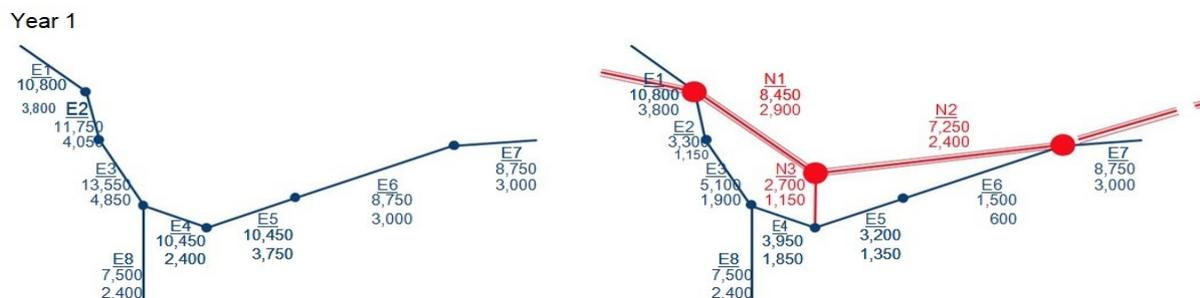
The traffic model was calibrated with traffic count data from 2012, and validity tests show that the model is sufficiently good in replicating the actual travel patterns. Future state matrices were multiplied by growth rates, which are based on assumed changes in population, economic activity, car ownership and transport cost. It was assumed that the traffic growth rate between 2017 and 2027 will be around 2 % per year, and around 1 %
