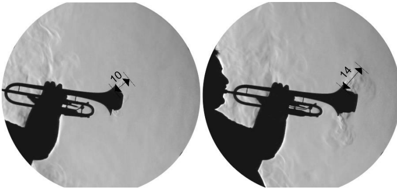
Figure 11 Maximal range of the air escaping from the bell with straight mute (left) and cup mute (right) [cm]
