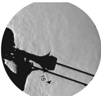
Figure 13 Maximal range of the air escaping from the bell with damper [cm]
