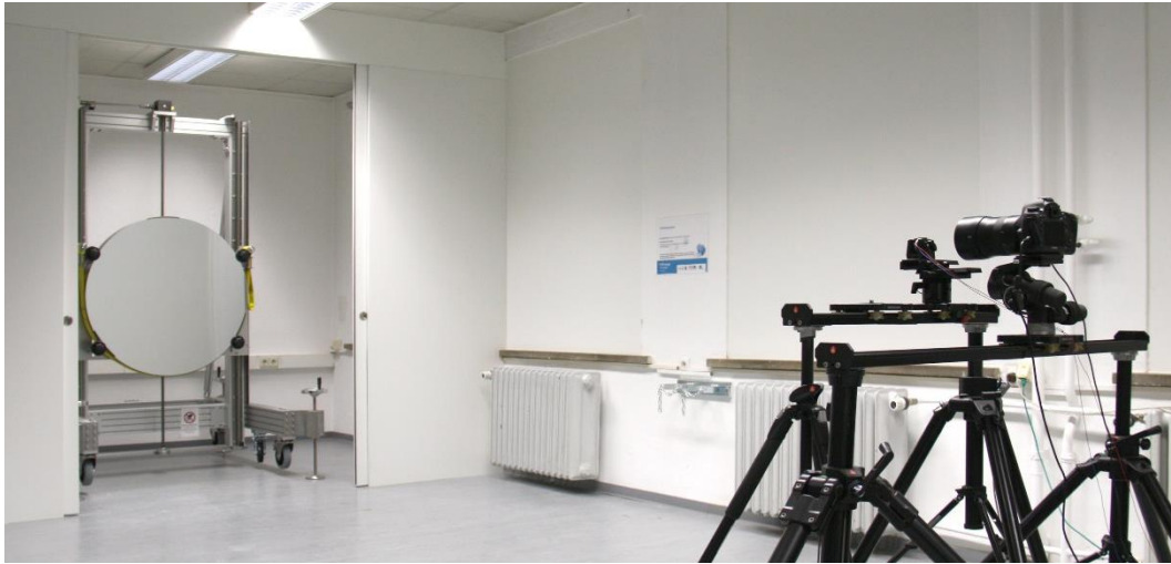
Figure 1 Experimental setup of the schlieren imaging system at the chair of Building Physics at the Bauhaus University Weimar, Germany
