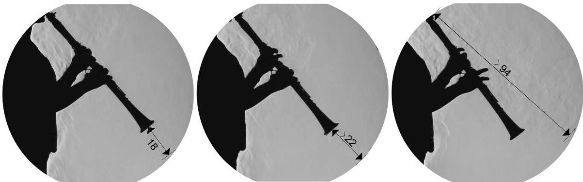
Figure 5 Bb clarinet in front of the schlieren mirror: maximal range of the air escaping from the bell while playing the note C#3 \approx 139 Hz (left), note E6 \approx 1319 Hz (center) and the air leaking at the mouthpiece (right) [cm]
