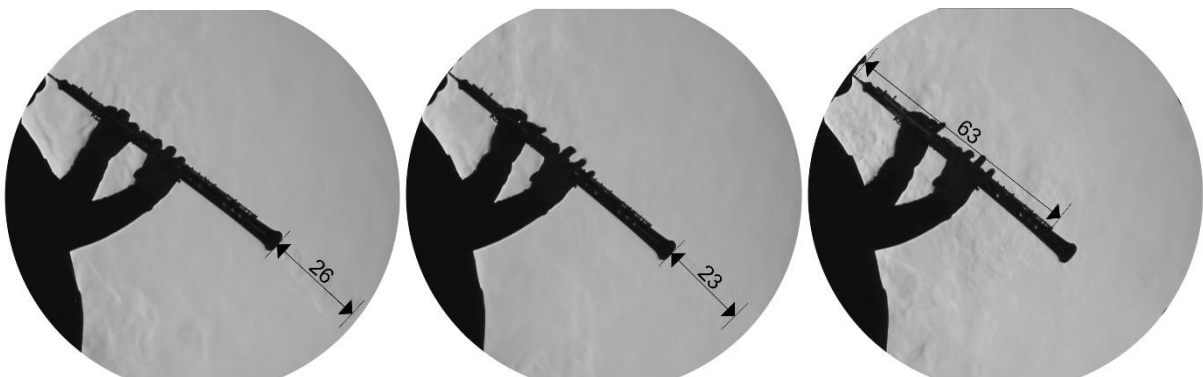
Figure 3 Oboe in front of the schlieren mirror: maximal range of the air escaping from the bell while playing the note Bb3 \approx 233 Hz (left), note D6 \approx 1175 Hz (center) and while intermittently exhaling (right) [cm] (cf. Richter et al. (2020))
