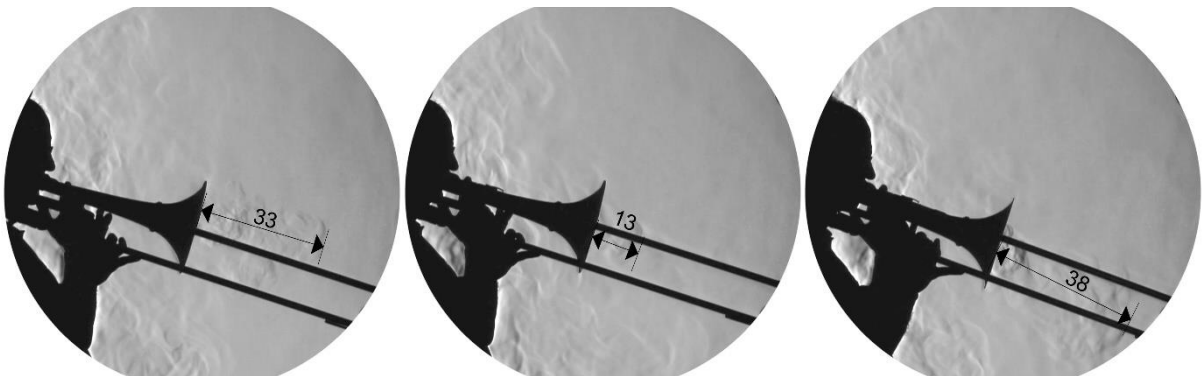
Figure 12 Tenor trombone in front of the schlieren mirror while playing the note Bb1 \approx 58 Hz (left), note Bb3 \approx 233 Hz (center) and the maximal range of the air escaping from the bell (right) [cm]
