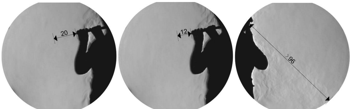
Figure 8 Piccolo flute in front of the schlieren mirror: maximal range of the air escaping from the foot joint while playing the note E_5 \approx 659 Hz (left), note G\#_7 \approx 3322 Hz (center) and the air blown above the mouthpiece (right) [cm]
