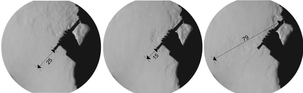
Figure 9 Soprano recorder in front of the schlieren mirror: maximal range of the air escaping from the bell while playing the note C5 \approx 523 Hz (left), note G6 \approx 1568 Hz (center) and the air escaping from the window (right) [cm]
