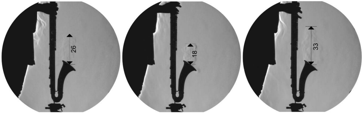
Figure 6 Bass clarinet in front of the schlieren mirror while playing the note D_2 \approx 73 Hz (left), note Bb_4 \approx 466 Hz (center) and the maximal range of the air escaping from the bell (right) [cm]
