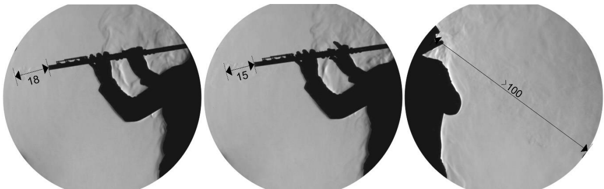
Figure 7 Traverse flute in front of the schlieren mirror: maximal range of the air escaping from the foot joint while playing the note E_4 \approx 330 Hz (left), note F_6 \approx 1397 Hz (center) and the air blown above the mouthpiece (right) [cm]
