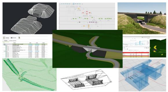
Figure 1: Overview of the partial models and partial results of the project (digital terrain model, alignment, earth work models, process map, marketing visualizations, quantity take-off, structural model, bridge model and finally, the overall coordination model in the middle).
