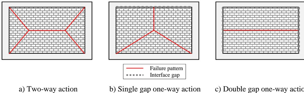
Figure 1: Failure modes depending on boundary conditions
